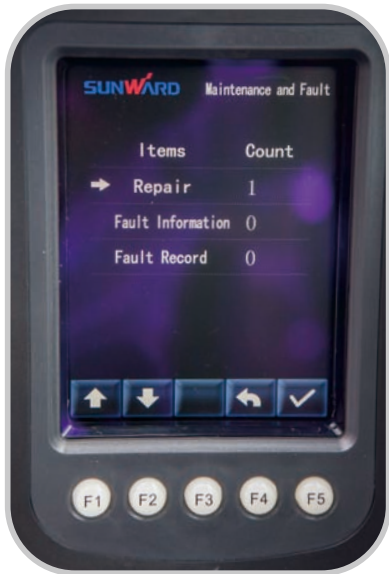
Maintenance and fault diagnosis
