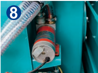
Fuel feed pump
